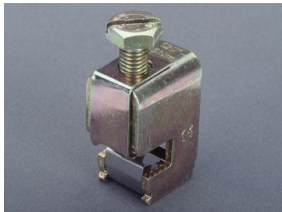
01 203 CRITO® universal conductor terminal for 10mm flat busbars 16 - 120 mm 2
