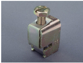
01 068 CRITO® universal conductor terminal for 5mm flat busbars 16 - 120 mm 2
